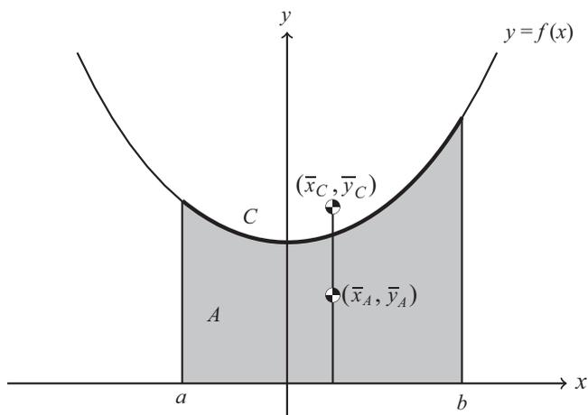
**Figure 1.** Two centroidal properties of the catenary (in standard vertical position)
