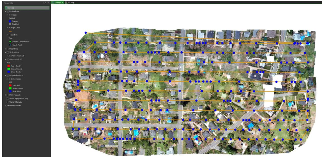
Figure 2. Drone2Map view site showing flight path and imagery points.
